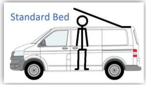
Standard Bed is single hinged and follows the same line up as the roof.
