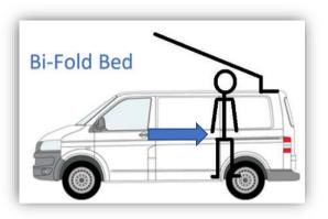
Bi-Fold Bed is double hinged and gives an additional 6/8 inches of head room towards the back of the van.
